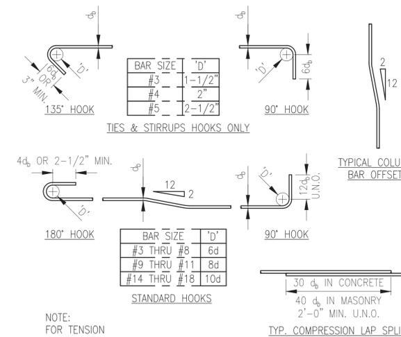
**3 TYP. REINF. BENDING DETAIL**
