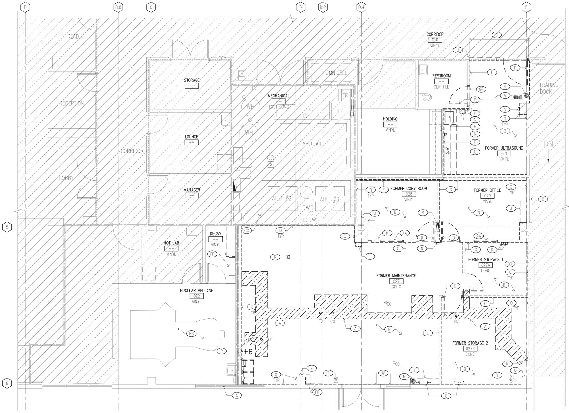
**1 DEMOLITION FLOOR PLAN - FORMER MAINTENANCE**
