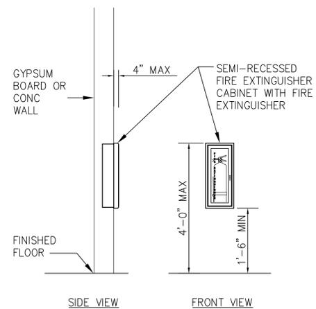
**7** FIRE EXTINGUISHER AND CABINET INSTALLATION DETAIL
