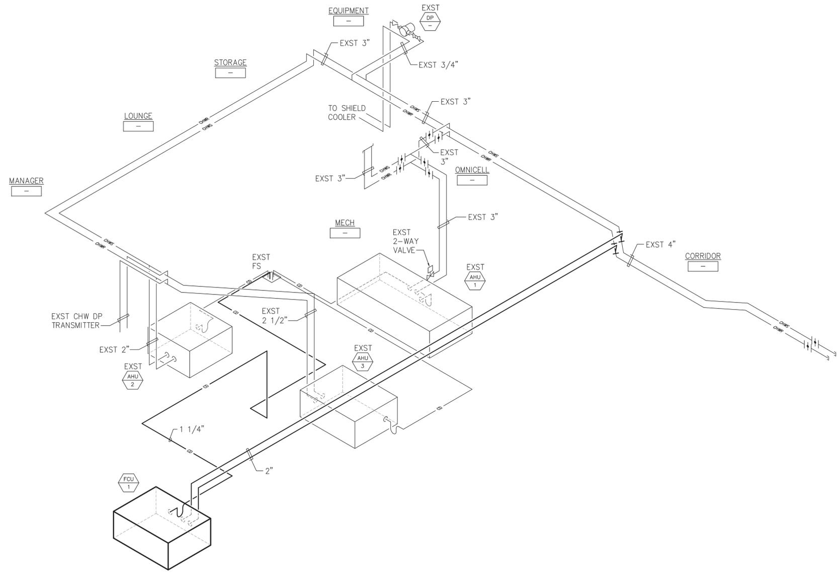
**CHILLED WATER PIPING DIAGRAM**
