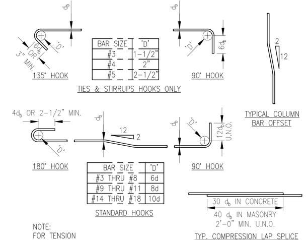
**3 TYP. REINF. BENDING DETAIL**
