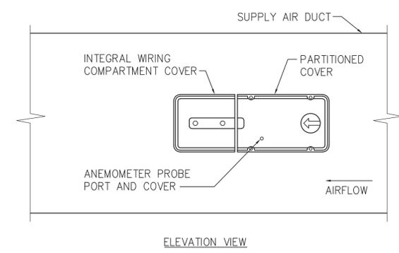
**7 DUCT DETECTOR DETAIL**
