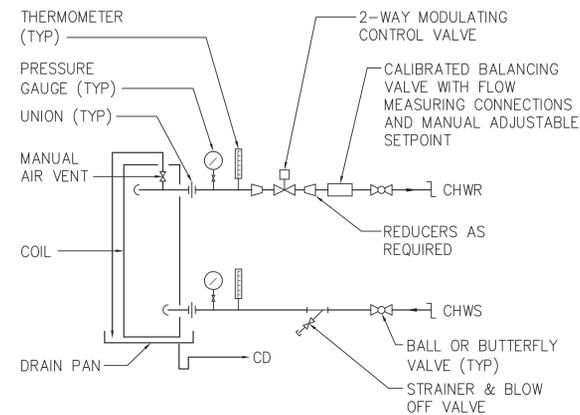
**3** AHU AND FCU CONNECTION DETAIL
