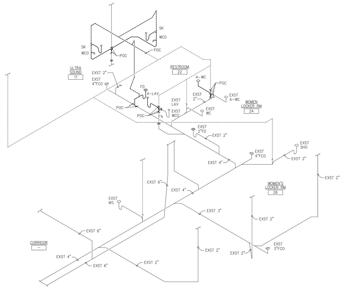
**SANITARY PIPING DIAGRAM – ULTRASOUND**
