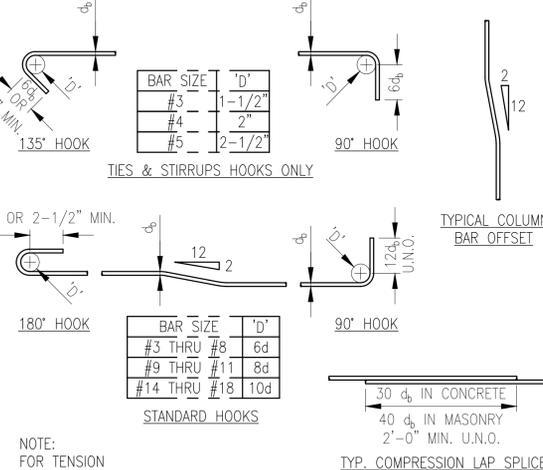
**3 TYP. REINF. BENDING DETAIL**
