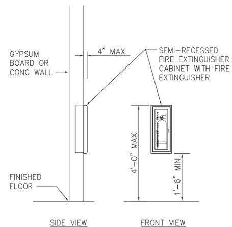
**7** FIRE EXTINGUISHER AND CABINET INSTALLATION DETAIL
