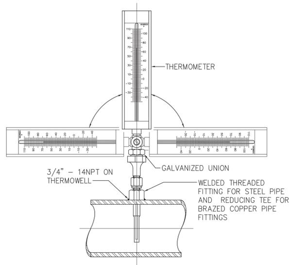
**1** ADJUSTABLE ANGLE THERMOMETER DETAIL
