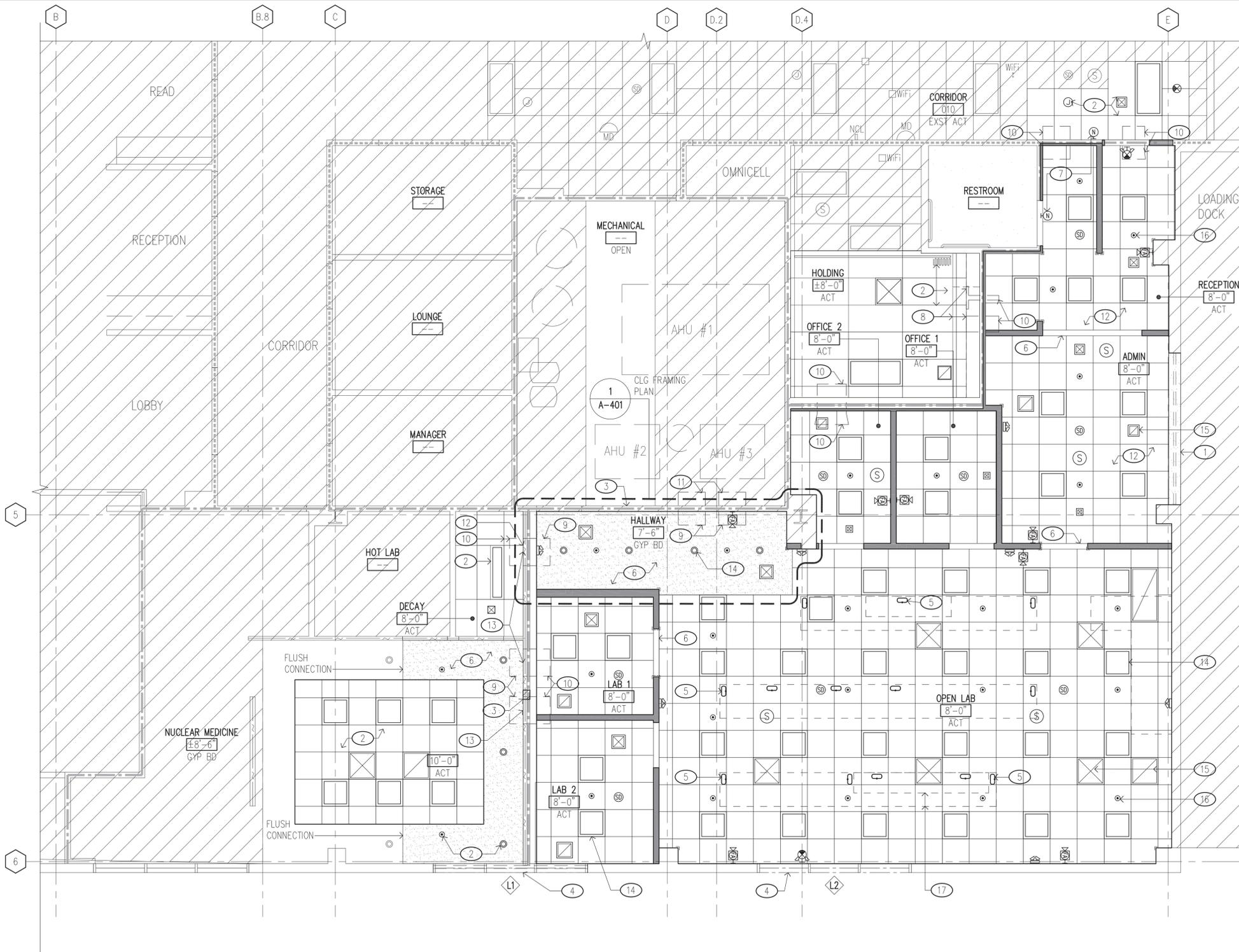
**1 REPAIR REFLECTED CEILING PLAN - LABORATORY**
