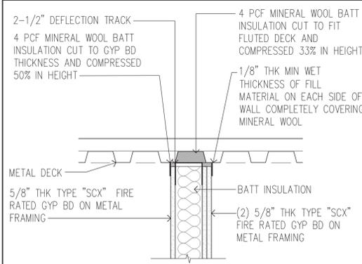
**8 FIRE RATED PARTITION DETAIL AT METAL DECK, TYP**
