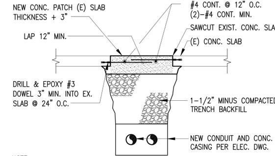
NOTE: WIDTH OF TRENCH TO BE FIELD DETERMINED AS NECESSARY TO PROPERLY INSTALL PROPOSED CONDUIT(S) & CASING
