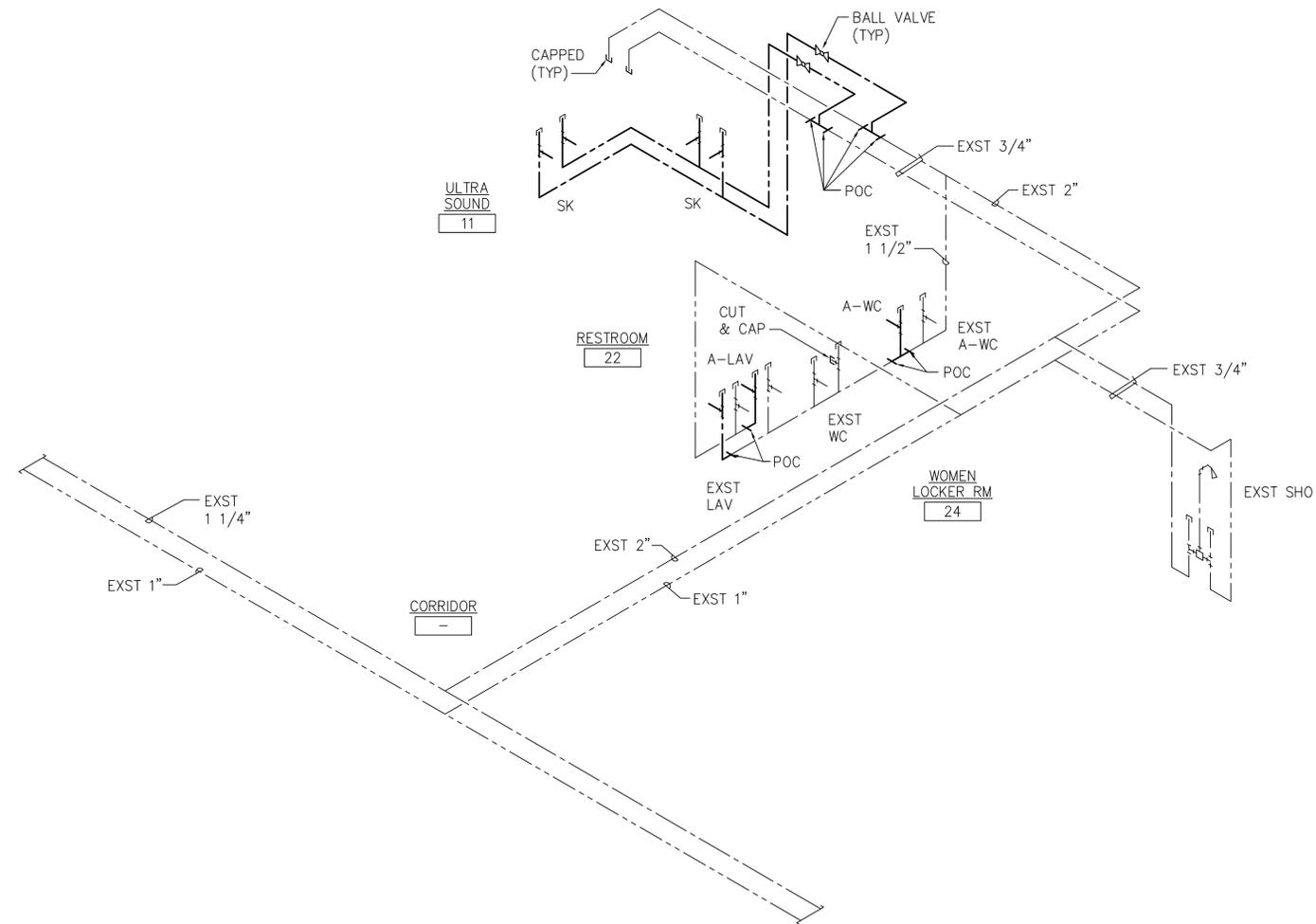
**WATER PIPING DIAGRAM – ULTRASOUND**
