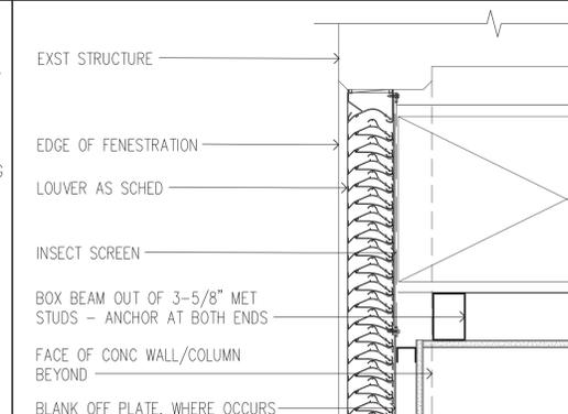
**9 GYP BD SOFFIT DETAIL AT NUCLEAR MED**
