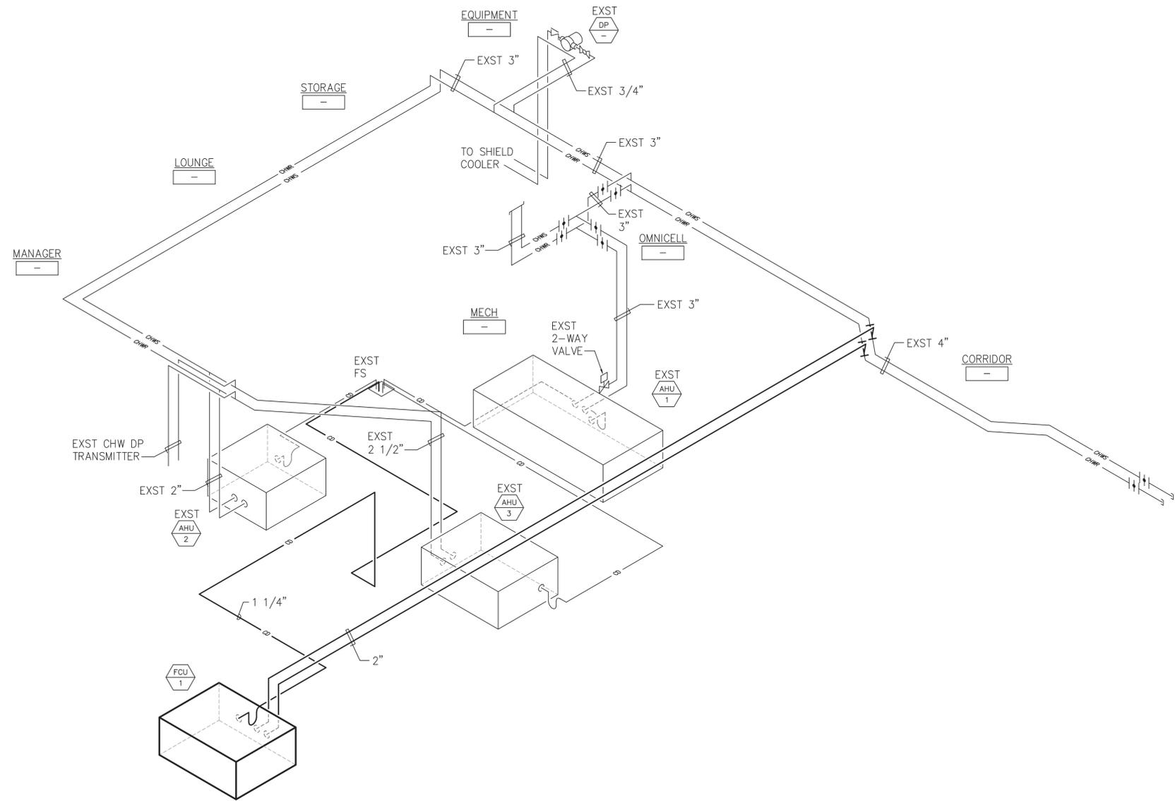
**CHILLED WATER PIPING DIAGRAM**
