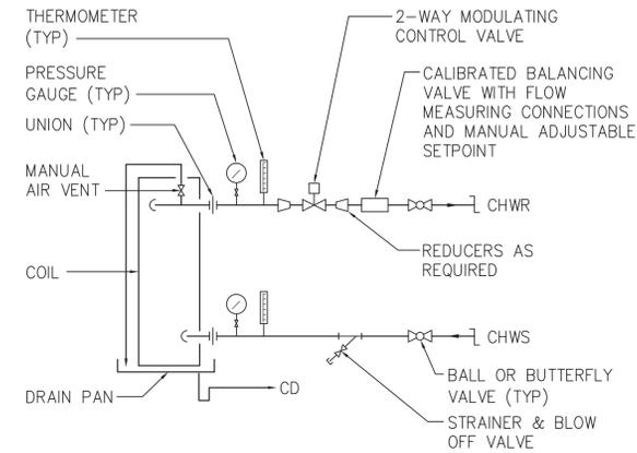
**3** AHU AND FCU CONNECTION DETAIL
