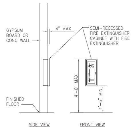
**7** FIRE EXTINGUISHER AND CABINET INSTALLATION DETAIL
