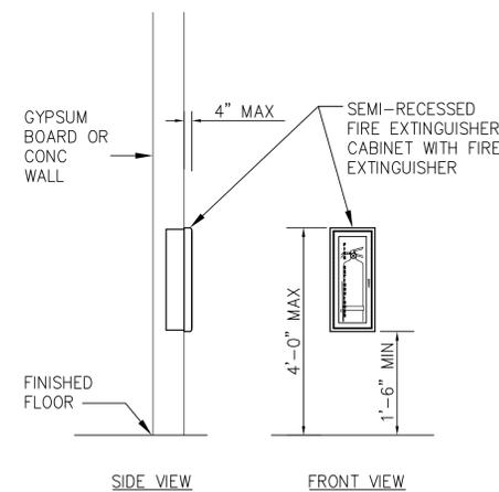
**7** FIRE EXTINGUISHER AND CABINET INSTALLATION DETAIL
