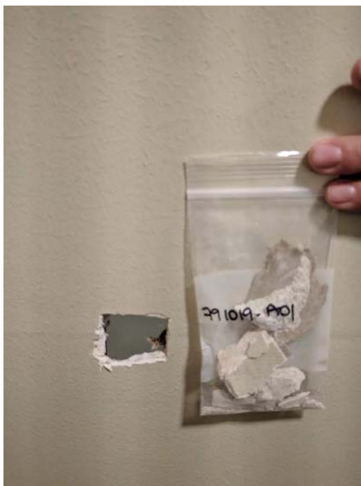
Photograph 02: Sampled drywall with joint compound & wall texture. Sample ID: 791019-A01
